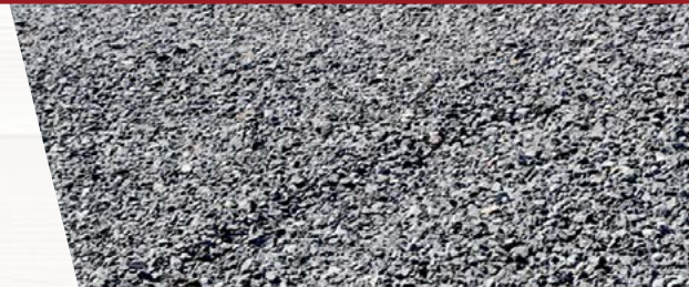
4-6" crushed limestone recommended for the pad
